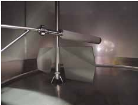
Aeration sintered tube and two-bladed agitator
