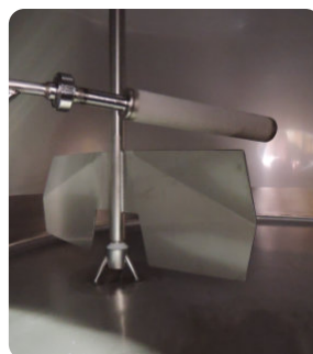
Aeration sintered tube and two-bladed agitator
