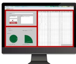
Create your own riddling programs with the Gyroprog® software (Windows® compatible). Once created, transfer the riddling program via a USB dongle in the Gyropalette® controller.
