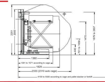
Loading/unloading by forklift with a minimum capacity of 1 200 kg
