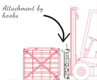
Forks up : single attachment by hooks for use with containers.
