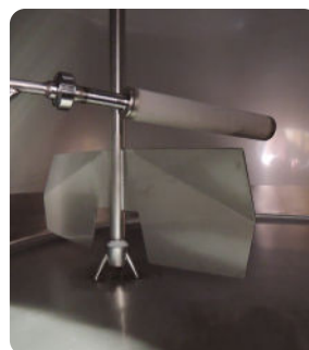
Aeration sintered tube and two-bladed agitator
